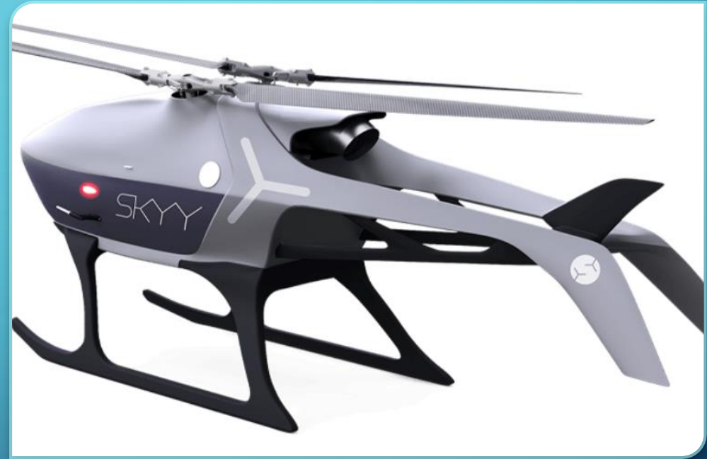
Skyy Avantia 100: 65kg Payload
